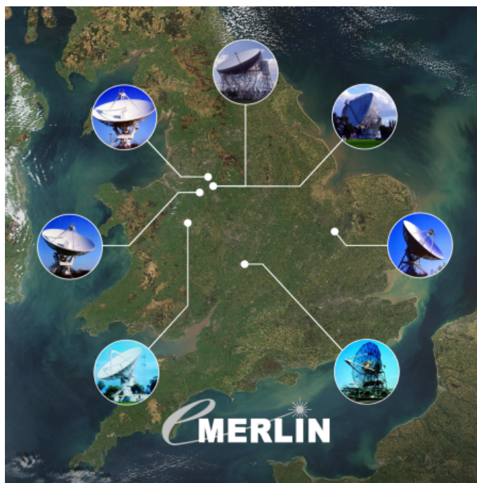
Figure 1.3: eMERLIN antennas over the map of the UK. The longest baseline is 217 km. Image from [16].
